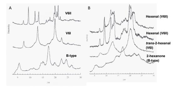
**Figure 2.** X-ray diffractogram of V6 structure (A) and amylose-flavour complexed (B) (Source: Jouquand *et al.*, 2006)
