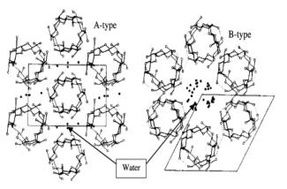
**Figure 4.** Crystalline packing of double helices in A-type and B-type of amylose (Source: Walter, 1998)
