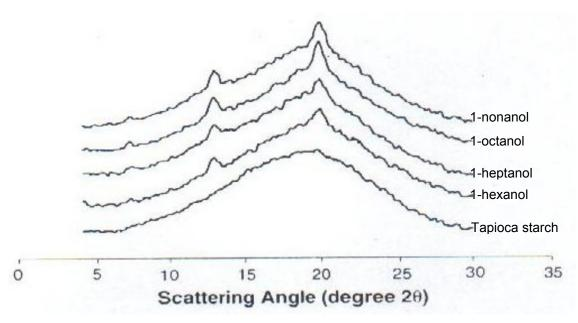
**Figure 3.** X-ray diffractogram of different tapioca-aliphatic alcohol complexes. (Source: Adapted from Itthisoponkul *et al.*, 2007)
